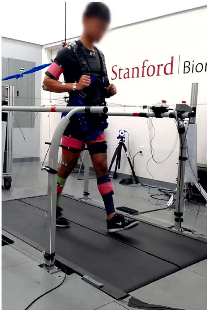
A participant walks on a treadmill while wearing motion capture markers, EMG sensors, and a safety harness, as part of a study using the 'Bump'em' perturbation robot to simulate real-world balance challenges.
